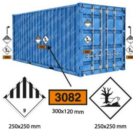
Example of Container transporting packaged dangerous goods of UN3082 loaded in excess of 4000 kg gross mass.<sup>5</sup>
